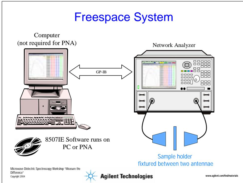
A typical freespace system consists of a vector network analyzer, two antennae facing each other with a sample holder between them. Agilent provides software that converts the reflection and transmission coefficients to dielectric properties. For the PNA series network analyzers, a computer is not required as the software can be run directly on the instrument.. For all other network analyzers, an external computer with HP-IB card is required.
