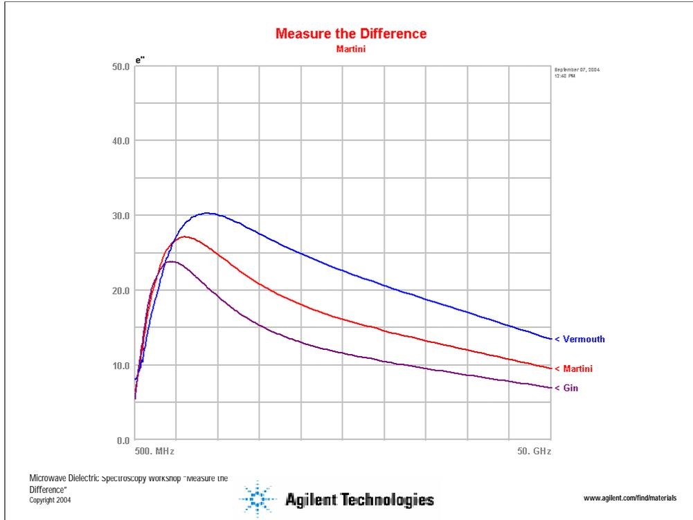
A martini is a mixture of gin and vermouth. Measuring the permittivity of this and other mixtures would allow you to determine the concentration of the mixture.
