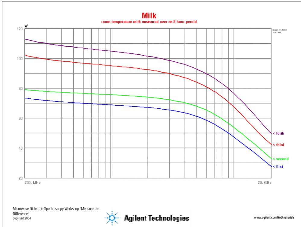
A glass of room temperature milk was measured over an eight hour period. The milk changed from being drinkable to spoiled. This suggests that bio-content can be correlated to dielectric properties.
