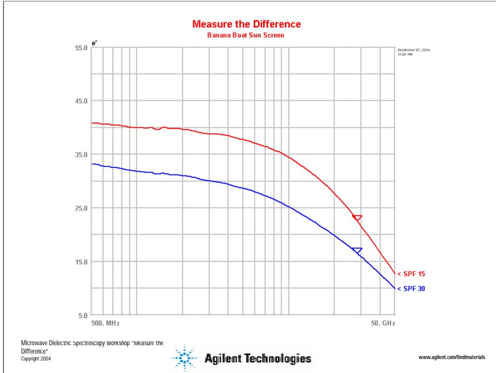
And just so you don't think that this measurement technique is only good for food products, here is a measurement of sun screen. The red trace is SPF15 and the blue trace is SPF30. Since microwave dielectric spectroscopy is not an optical technique it does not have problems measuring opaque or white materials.
