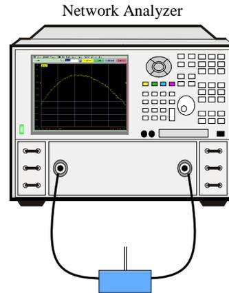
Resonant Cavity with sample connected between ports.
