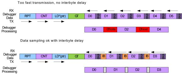
Figure 33-18. Interbyte Delay Example with LD and RPT
