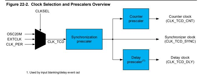
The TCD synchronizer clock is separate from the other module clocks enabling faster synchronization between the TCD domain and the I/O domain. The total prescaling for the counter is:
