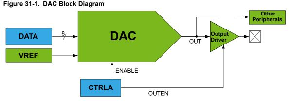
**Note:** Only DAC0 has an output driver for an external pin.
