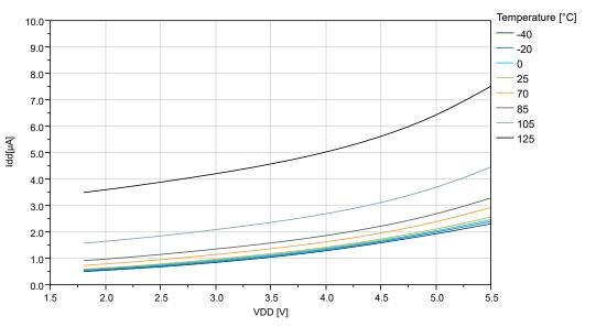
Figure 38-13. ATtiny1616 Standby Mode Supply Current vs. V<sub>DD</sub> (RTC Running with Internal OSCULP32K)
