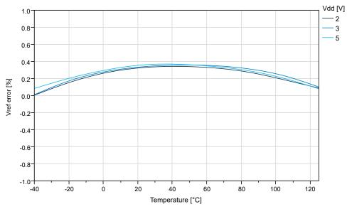
Figure 38-45. Internal 0.55V Reference vs. Temperature
