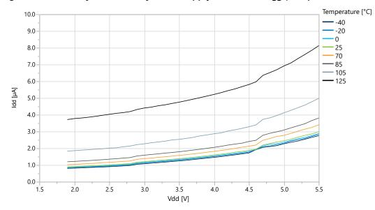
Figure 38-27. ATtiny3216 Standby Mode Supply Current vs. V<sub>DD</sub> (Sampled BOD Running at 1 kHz)
