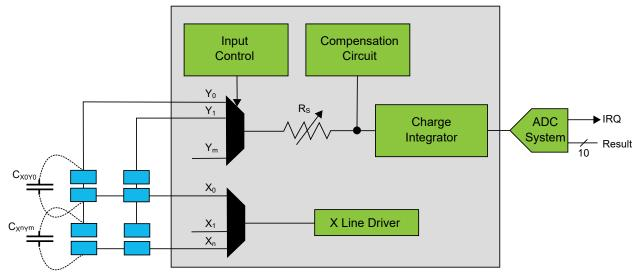
Figure 32-2. PTC Block Diagram Self Capacitance
