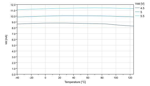
Figure 38-3. ATtiny1616 Active Supply Current vs. Temperature (f=20 MHz OSC20M)
