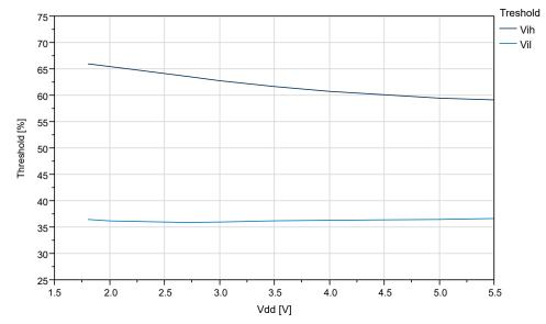
Figure 38-31. I/O Pin Input Threshold Voltage vs. V<sub>DD</sub> (T=25°C)
