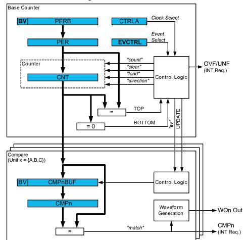
Figure 20-2. Timer/Counter Block Diagram
