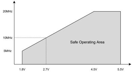
Figure 37-1. Maximum Frequency vs. V<sub>DD</sub> for [-40, 105]°C
