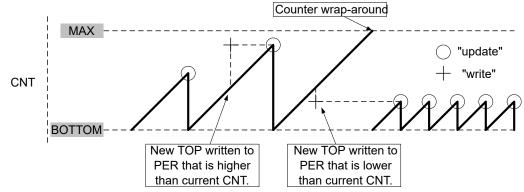
A counter wrap-around can occur in any mode of operation when up-counting without buffering. This is due to the fact that the TCAn.CNT and TCAn.PER registers are continuously compared: if a new TOP value is written to TCAn.PER that is lower than the current TCAn.CNT, the counter will wrap first, before a compare match happens.
