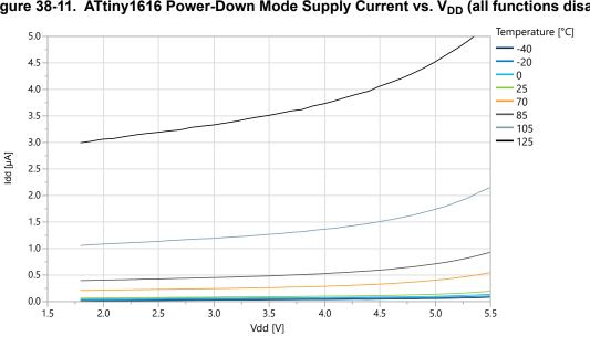
Figure 38-11. ATtiny1616 Power-Down Mode Supply Current vs. V<sub>DD</sub> (all functions disabled)
