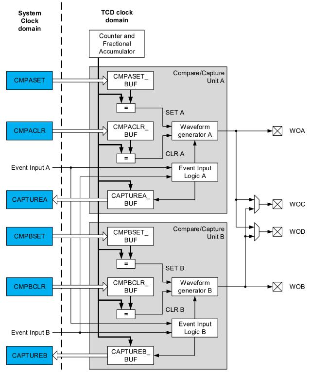
The TCD core is asynchronous to the system clock. The timer/counter consist of two compare/capture units, each with a separate waveform output. In addition, there are two extra waveform outputs which can be equal to the output from one of the units. The compare registers CMPxSET and CMPxCLR are stored
