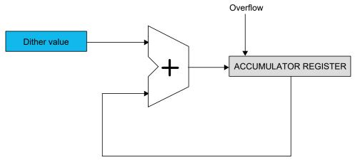
The user can select where in the TCD cycle the Dither will be added by writing to the Dither Selection bits in the Dither Control register (DITHERSEL in TCDn.DITCTRL):
