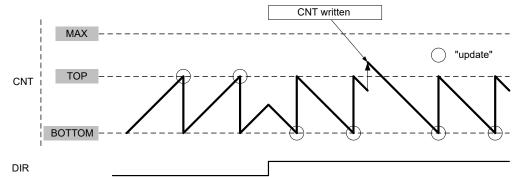
It is possible to change the counter value in the Counter register (TCAn.CNT) when the counter is running. The write access to TCAn.CNT has higher priority than count, clear, or reload, and will be immediate. The direction of the counter can also be changed during normal operation by writing to DIR in TCAn.CTRLE.
