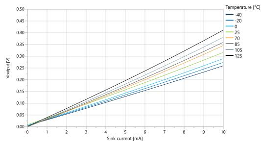
Figure 38-35. I/O Pin Output Voltage vs. Sink Current (V<sub>DD</sub>=3.0V)
