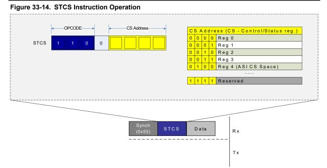
Figure 33-14 shows the data frame transmitted after the SYNCH and instruction frames. There is no response generated from the STCS instruction, as is the case for ST and STS.
