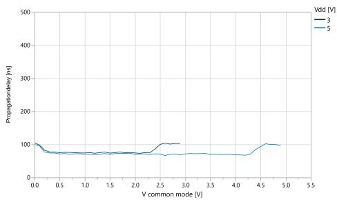
Figure 38-70. Propagation Delay vs.  $V_{CM}$  LPMODE Enabled, Rising Positive Input,  $V_{OD}$  = 30 mV (T=25°C)
