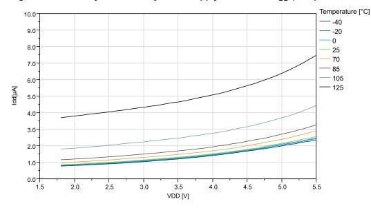
Figure 38-15. ATtiny1616 Standby Mode Supply Current vs. V<sub>DD</sub> (Sampled BOD Running at 1 kHz)
