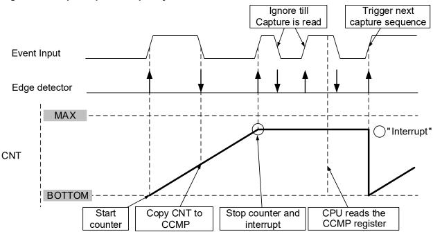
Figure 21-7. Input Capture Frequency and Pulse-Width Measurement
