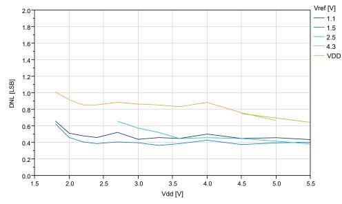
Figure 38-58. DNL vs. V<sub>ref</sub> (V<sub>DD</sub>=5.0V, f<sub>ADC</sub>=115 ksps), REFSEL = Internal Reference
