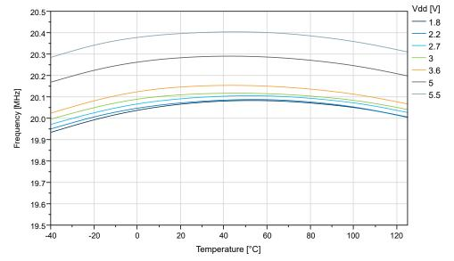
Figure 38-75. OSC20M Internal Oscillator: Frequency vs. Temperature
