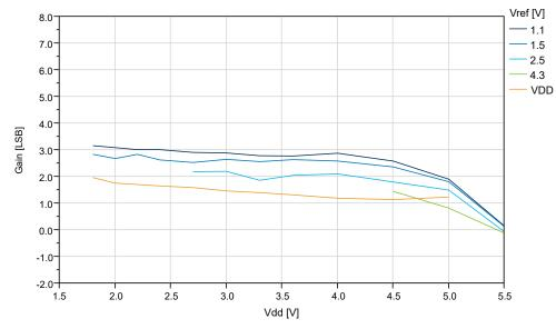
Figure 38-60. Gain Error vs. V<sub>ref</sub> (V<sub>DD</sub>=5.0V, f<sub>ADC</sub>=115 ksps), REFSEL = Internal Reference
