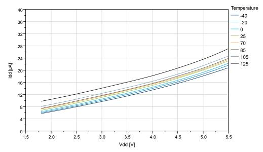
Figure 38-5. ATtiny1616 Active Supply Current vs. V<sub>DD</sub> (f=32 KHz OSCULP32K)
