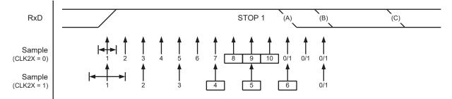
A new high-to-low transition indicating the Start bit of a new frame can come right after the last of the bits used for majority voting. For Normal-Speed mode, the first low-level sample can be at the point marked (A) in Stop Bit Sampling and Next Start Bit Sampling. For Double-Speed mode, the first low level must be delayed to point (B). Point (C) marks a Stop bit of full length at the nominal baud rate. The early Start bit detection influences the operational range of the receiver.
