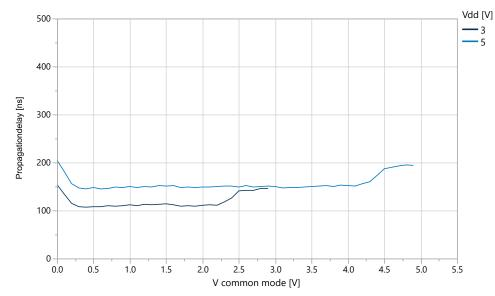
Figure 38-71. Propagation Delay vs.  $V_{CM}$  LPMODE Disabled, Falling Positive Input,  $V_{OD}$  = 30 mV (T=25°C)
