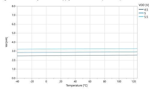
Figure 38-23. ATtiny3216 Idle Supply Current vs. Temperature (f=20 MHz OSC20M)
