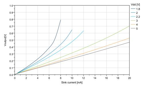
Figure 38-37. I/O Pin Output Voltage vs. Sink Current (T=25°C)
