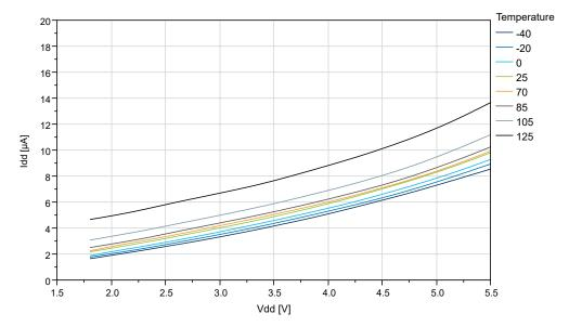
Figure 38-9. ATtiny1616 Idle Supply Current vs. V<sub>DD</sub> (f=32 KHz OSCULP32K)
