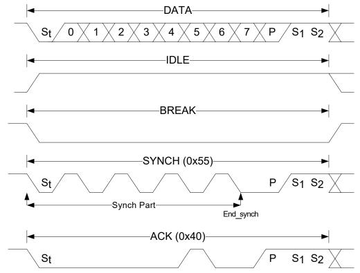
DataData frame consists of one Start bit (always low), eight data bits, one parity bit (even parity),Frameand two Stop bits (always high). If the Start bit, parity bit, or Stop bits have an incorrect value,<br/>an error will be detected and signalized by the UPDI. The parity bit-check in the UPDI can be<br/>disabled by writing the PARD bit in UPDI.CTRLA, in which case the parity generation from the<br/>debugger can be ignored.
