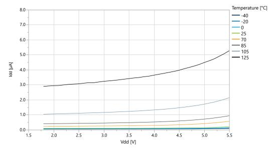
Figure 38-29. ATtiny3216 Power-Down Mode Supply Current vs. V<sub>DD</sub> (all functions disabled)
