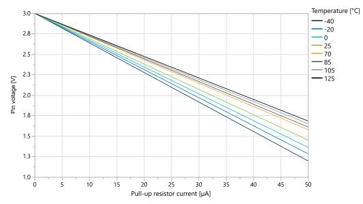
Figure 38-43. I/O Pin Pull-Up Resistor Current vs. Input Voltage (V<sub>DD</sub>=3.0V)
