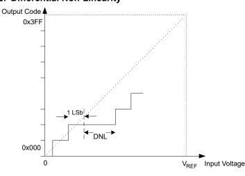
**Quantization Error** Due to the quantization of the input voltage into a finite number of codes, a range of input voltages (1 LSb wide) will code to the same value. Always ±0.5 LSb.
