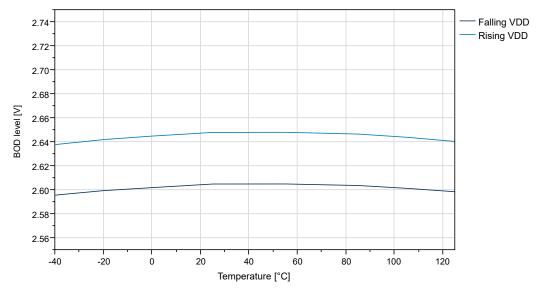
Figure 38-54. BOD Threshold vs. Temperature (Level 4.3V)
