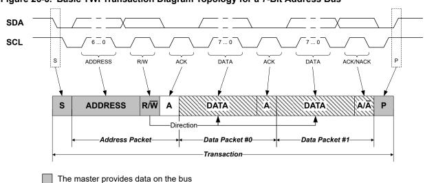
Figure 26-3. Basic TWI Transaction Diagram Topology for a 7-Bit Address Bus
