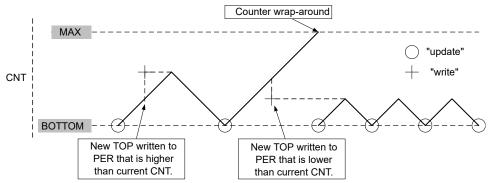
**With Buffering:** When double buffering is used, the buffer can be written at any time and still maintain correct operation. The TCAn.PER is always updated on the UPDATE condition, as shown for dual-slope operation in the figure below. This prevents wrap-around and the generation of odd waveforms.
