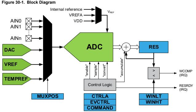
The analog input channel is selected by writing to the MUXPOS bits in the MUXPOS register (ADC.MUXPOS). Any of the ADC input pins, GND, or temperature sensor, can be selected as singleended input to the ADC. The ADC is enabled by writing a '1' to the ADC ENABLE bit in the Control A register (ADC.CTRLA). Voltage reference and input channel selections will not go into effect before the ADC is enabled. The ADC does not consume power when the ENABLE bit in ADC.CTRLA is '0'.
