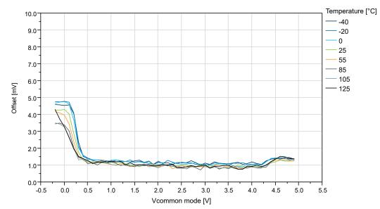
Figure 38-67. Offset vs.  $V_{CM}$  - 10 mV ( $V_{DD}$ =5V)
