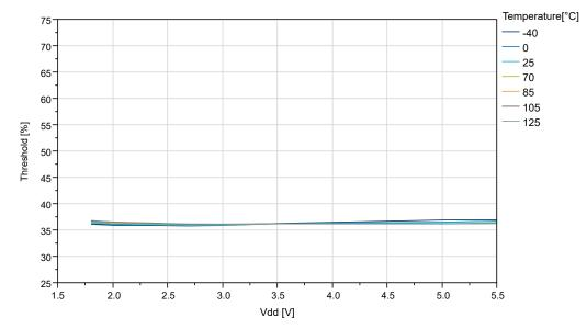
Figure 38-33. I/O Pin Input Threshold Voltage vs.  $V_{DD}$  (V<sub>IL</sub>)
