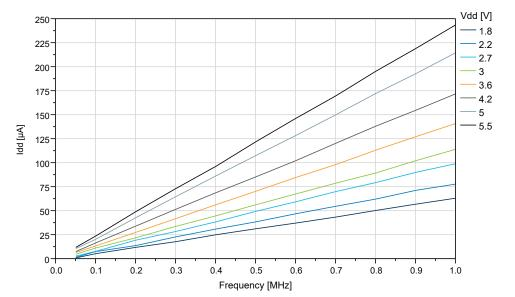
Figure 38-7. ATtiny1616 Idle Supply Current vs. Low Frequency (0.1-1.0 MHz) at T=25°C
