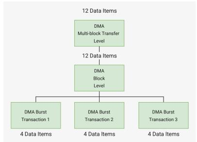
If the DW\_apb\_ssi makes a transmit request to this channel, four data items are written to the DW\_apb\_ssi transmit FIFO. Similarly, if the DW\_apb\_ssi makes a receive request to this channel, four data items are read from the DW\_apb\_ssi receive FIFO. Three separate requests must be made to this DMA channel before all 12 data items are written or read.
