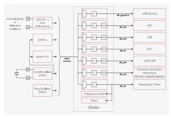
For very low cost or low power applications where precise timing is not required, the chip can be run from the internal Ring Oscillator (ROSC). Alternatively the user can provide external clocks or construct simple relaxation oscillators
