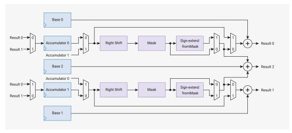
The processor can write or read any interpolator register in one cycle, and the results are ready on the next cycle. The processor can also perform an addition on one of the two accumulators ACCUMO or ACCUMO by writing to the corresponding ACCUMX\_ADD register.
