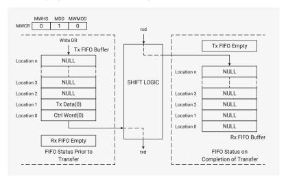
Continuous transfers occur as shown in Figure 142, with the control word for the next transfer following immediately after the LSB of the current data word.
