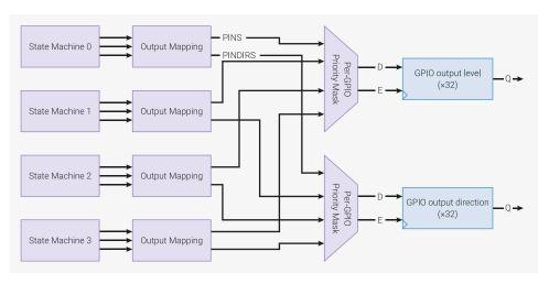
Each state machine may assert an OUT/SET and a side-set through its pin mapping hardware on each cycle. This generates 32 bits of write data and write mask for the GPIO output level and output enable registers, from each state machine.
