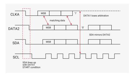
Control of the bus is determined by address or master code and data sent by competing masters, so there is no central master nor any order of priority on the bus.
