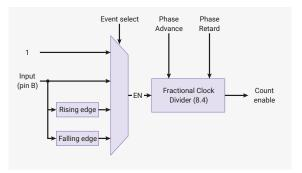
By default, each slice's counter is free-running, and will count continuously whenever the slice is enabled. There are three other options available:
