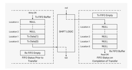
For receive only transfers (transfer mode field (9:8) of the Control Register 0 = 10b), data transmitted from the DW\_apb\_ssi to the external serial device is invalid, so a single dummy word is written into the transmit FIFO to begin the serial transfer. The txd output from the DW\_apb\_ssi is held at a constant logic level for the duration of the serial transfer. Data received from the external serial device into the DW\_apb\_ssi is pushed into the receive FIFO.
