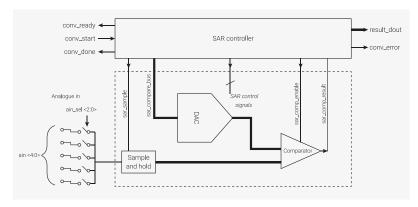
The ADC requires a 48MHz clock (clk\_adc), which could come from the USB PLL. Capturing a sample takes 96 clock cycles (96 × 1/48MHz) = 2µs per sample (500ksps). The clock must be set up correctly before enabling the ADC.
