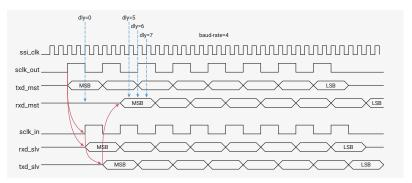
The Slave uses the sclk\_out signal from the master as a strobe in order to drive rxd signal data onto the serial bus. Routing and sampling delays on the sclk\_out signal by the slave device can mean that the rxd bit has not stabilized to the correct value before the master samples the rxd signal. Figure 121 shows an example of how a routing delay on the rxd signal can result in an incorrect rxd value at the default time when the master samples the port.
