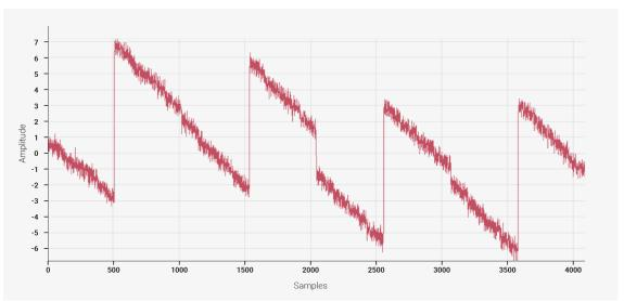
Nominally an ADC moves from one digital value to the next digital value, colloquially expressed as "no missing codes". However, if the ADC skips a value bin this would cause a spike in the Differential Non-Linearity (DNL) error. These types of error often only occur at specific codes due to the design of the ADC.
