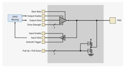
The pad's Output Enable, Output Data and Input Data ports are connected, via the IO mux, to the function controlling the pad. All other ports are controlled from the pad control register. The register also allows the pad's output driver to be disabled, by overriding the Output Enable signal from the function controlling the pad. See GPIO0 for an example of a pad control register.
