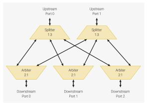
The crossbar is built from two components:
